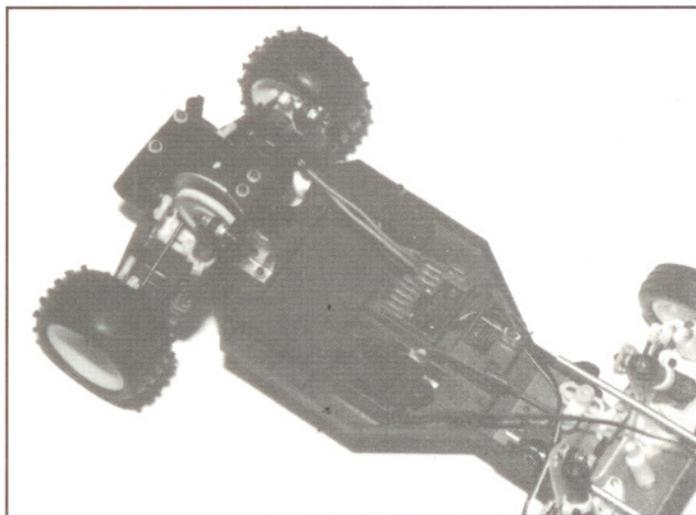
Thank you for your purchase of the TEKIN Active-Link Suspension chassis. This is the most technologically advanced replacement chassis ever offered for the Associated RC10 and RC10T. The unique design of the chassis and suspension components maximize performance by increasing the contact patch of the rear tires in all racing situations. The result is better-than-ever traction on any type of surface.
