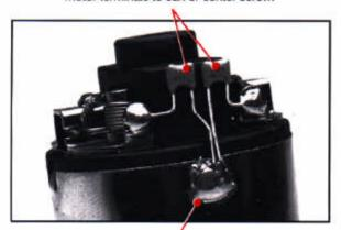
Scrape away paint or finish before soldering to the motor can.
