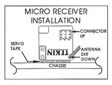
steady. If it does not, then you will need to move the receiver and/or motor wires around in the car. Do not run a large battery power wire near the receiver. You may need to install the receiver on its side. Tekin receivers are highly recommended. They should be installed on their side with the plugs up and the antenna and crystal down.
