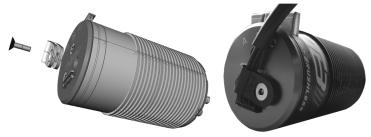
Drill .120" holes to fit #4 screws supplied
