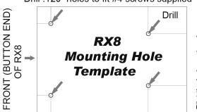
Pilot the holes out and ensure proper alignment.
