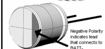
Negative Polarity indicates lead that connects to BATT-
